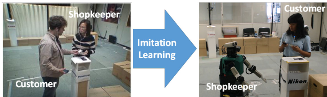
Figure 2. Natural human-human interaction data is collected with a passive sensor network and used to train a robot to replace the target human (e.g. a camera shopkeeper) [8,11].
